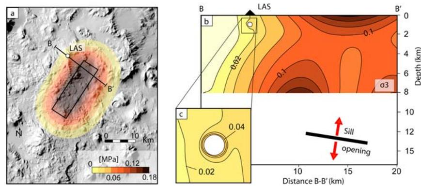
**Figure 3.** Stress transfer model at Lazufre for the period from 1997 to 2000. Maximum tensile stress  $\sigma_3$  is caused in the area of interest by the deep source inflation (a) at the surface. The rectangle represents the best fit dislocation plane projected to the surface, (b and c) cross-section through B – B' that shows a slight increase of the tensile stress around the simulated source of Lastarria volcano.
