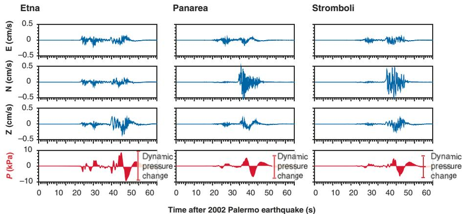
**Figure 3. Synthetic seismograms showing east-west (E), north-south (N), and vertical components (Z). From these three components, we determined the pressure change (P, shown in red) as function of time. Pressure fluctuations reached  $\pm 10$  kPa for Mount Etna and  $\pm 8$  kPa for the Panarea and Stromboli Island volcanoes.**
